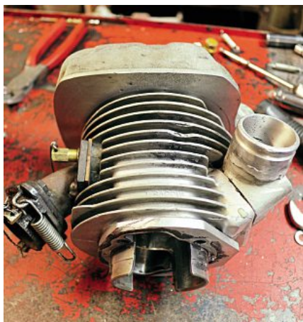
The entire top end of the engine removed as one unit as sealants were set solid, now that's airtight!
