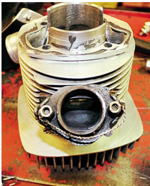
Packer plate at cylinder base for the long crank rod. Exhaust nuts securely lock-wired.
