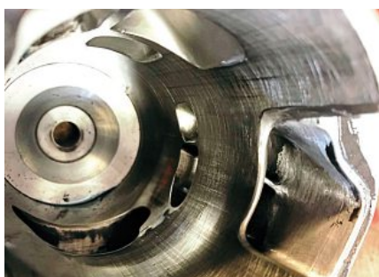
Even the packer plate is carefully ported to match the cylinder and case, for maximum flow.
