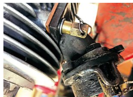
Chalky's own exhaust stub 'bridge' can be seen here from the side, between the cylinder and stub.
