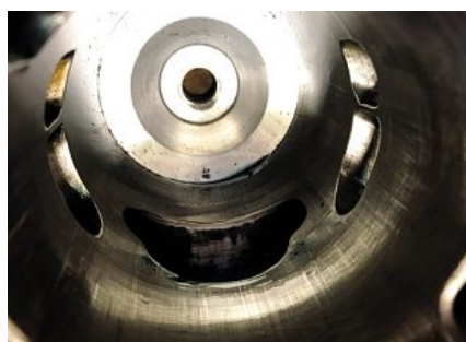
Porting arrangement can be seen clearly, with the popular 'chef's hat' style exhaust port shape.
