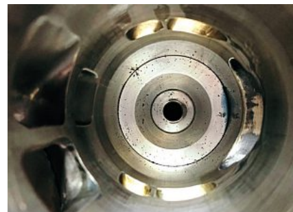
Centre plug, centre squish head. 128° transfer and 197° exhaust.
