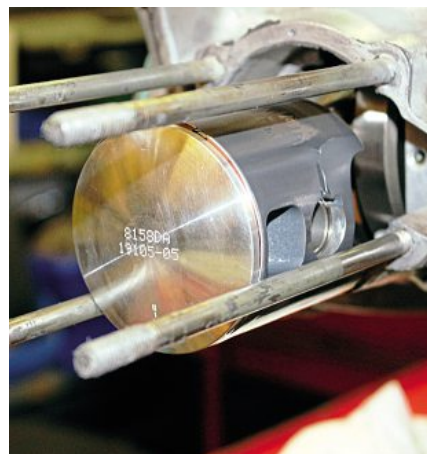
Lightweight Wossner/Suzuki piston with heat coating – despite being part of a race-winning engine, it almost looks brand new.
