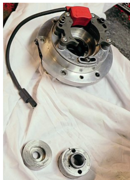
The diminutive Selettra ignition system components... now that's what I call a lightweight ignition!
