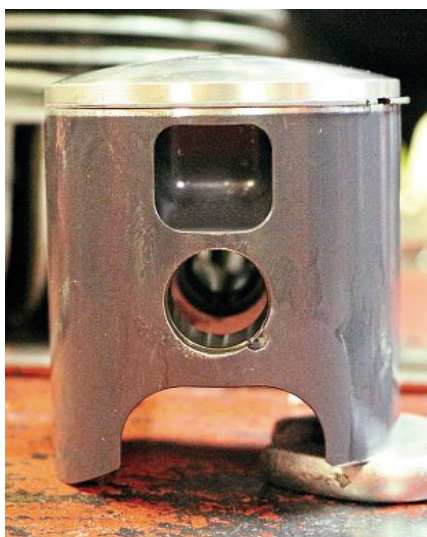
The painstakingly trimmed skirt brings the engine's inlet timing to near 200° for some tracks.
