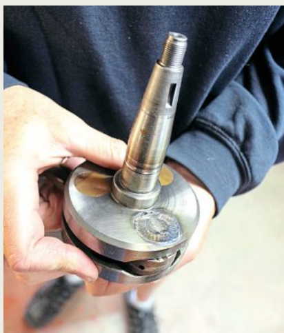
Even with a tight fit and weld on the pin, this crank started to spread.
