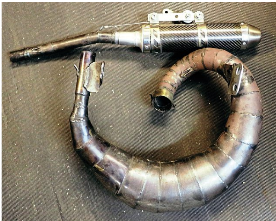
PipeDesign Hornet exhaust, routed to Chalky's own design spec, mounting brackets altered, and completed with carbon end can.
