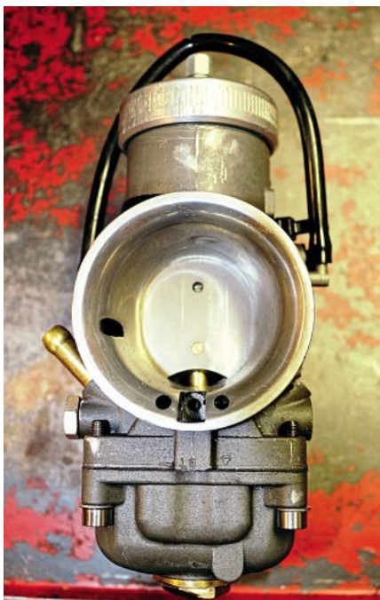
39mm Dellorto race carb, a large unit for a small motor, but ensures maximum peak power.
