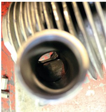
This close-up shot shows how the inlet manifold has been painstakingly flowed and matched by Chalky.
